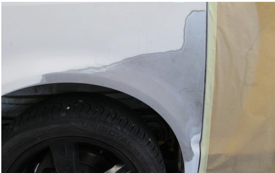
Picture 13: Volkswagen T5 (built 2013) with repaired right side panel – Delivery condition achieved with application of 2K epoxy resin body filler.
