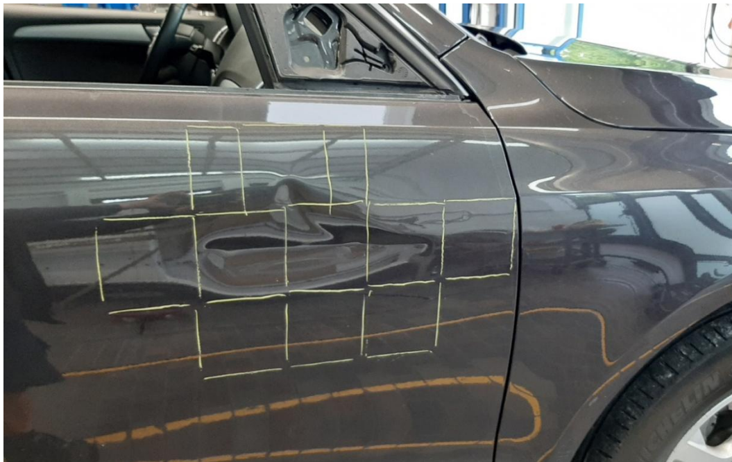
Picture 8: Damaged area as given to the repair shop – example 3.
