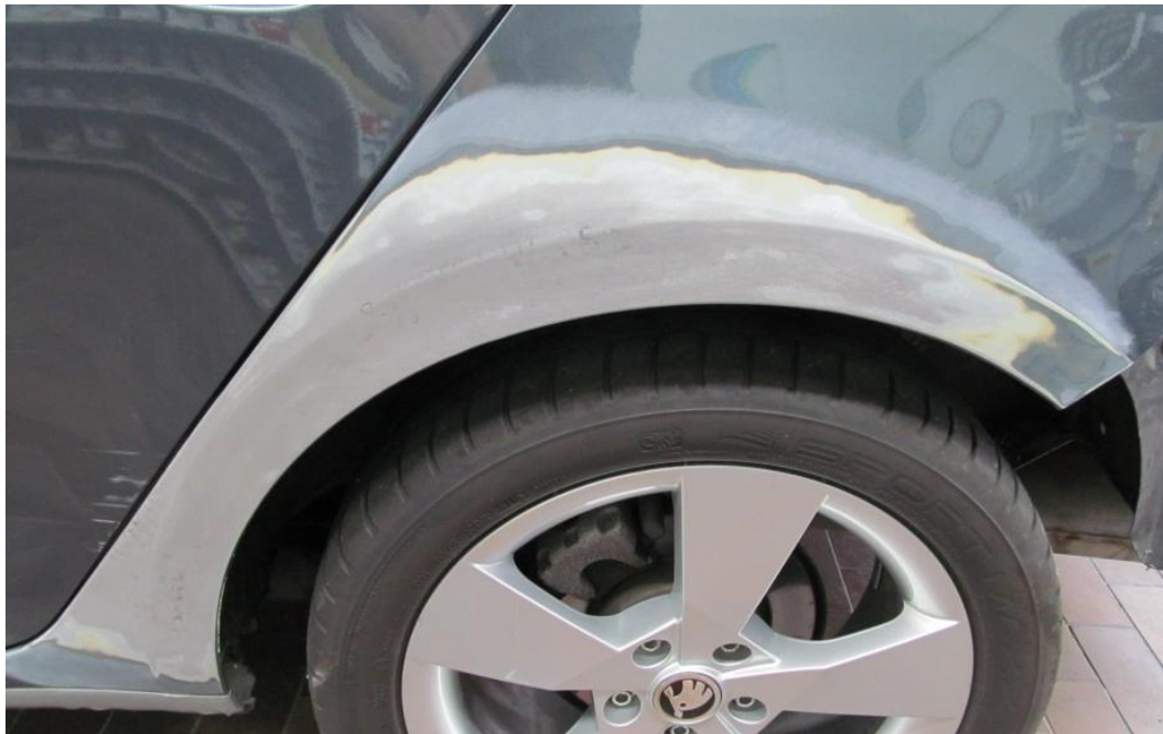
Picture 12: Skoda Octavia (5E; built 2015) with repaired left side panel – Delivery condition achieved without application of 2K epoxy resin body filler but with sheet metal repair only.
