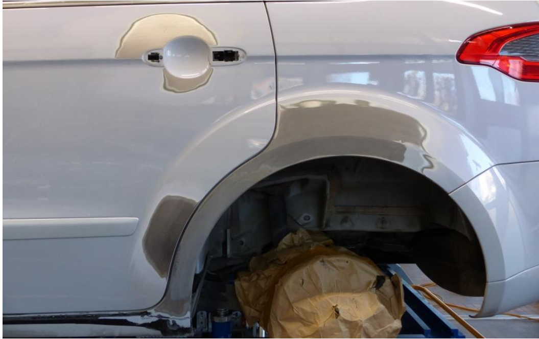
Picture 14: Ford S-Max (WA6; built 2012) with repaired left rear door (without body filler) and left side panel (including application of 2K epoxy resin body filler).
