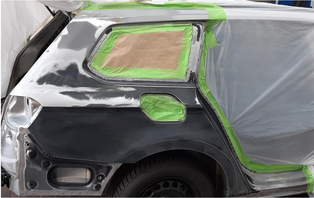
Picture 16: Replaced right side panel (welded in part) on a VW Passat (B8; built 2015) – Delivery condition achieved with application of 2K epoxy resin body filler.
