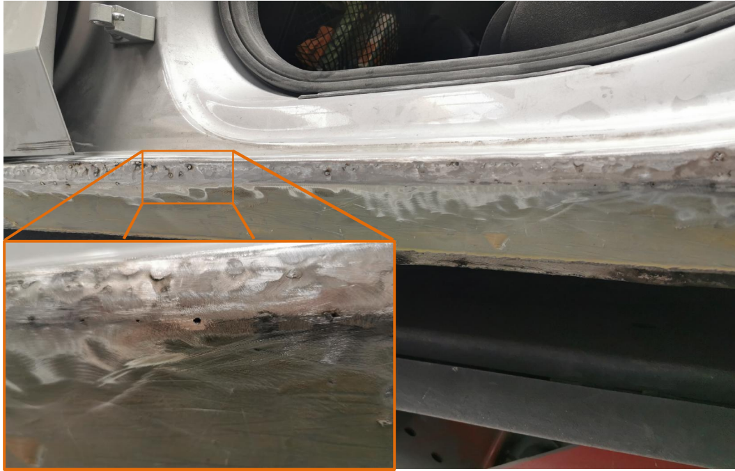
Picture 18: Delivery condition not achieved due to non-welded holes in the sheet metal, lack of final sheet metal treatment or application of body filler, high roughness due to missing final grinding and missing smooth transition area to the existing paint.
