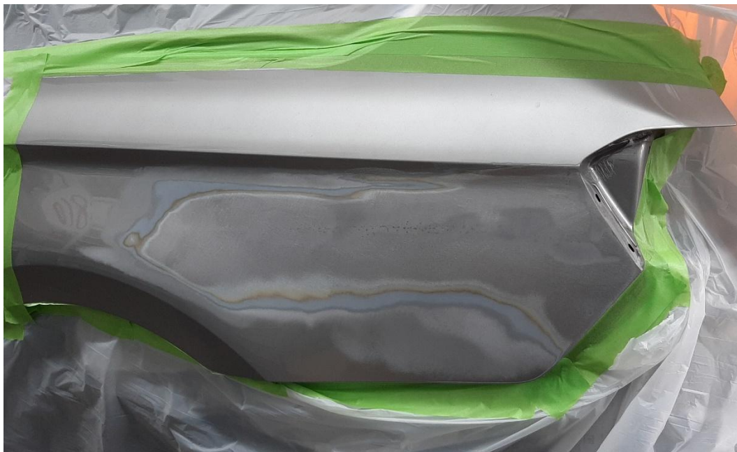
Picture 15: VW Passat (B8; built 2015) with repaired left side panel – Delivery condition achieved with application of 2K epoxy resin body filler.
