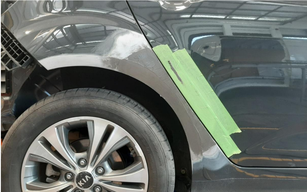
Picture 6: Application of 2K epoxy resin body filler after sheet metal repair.
