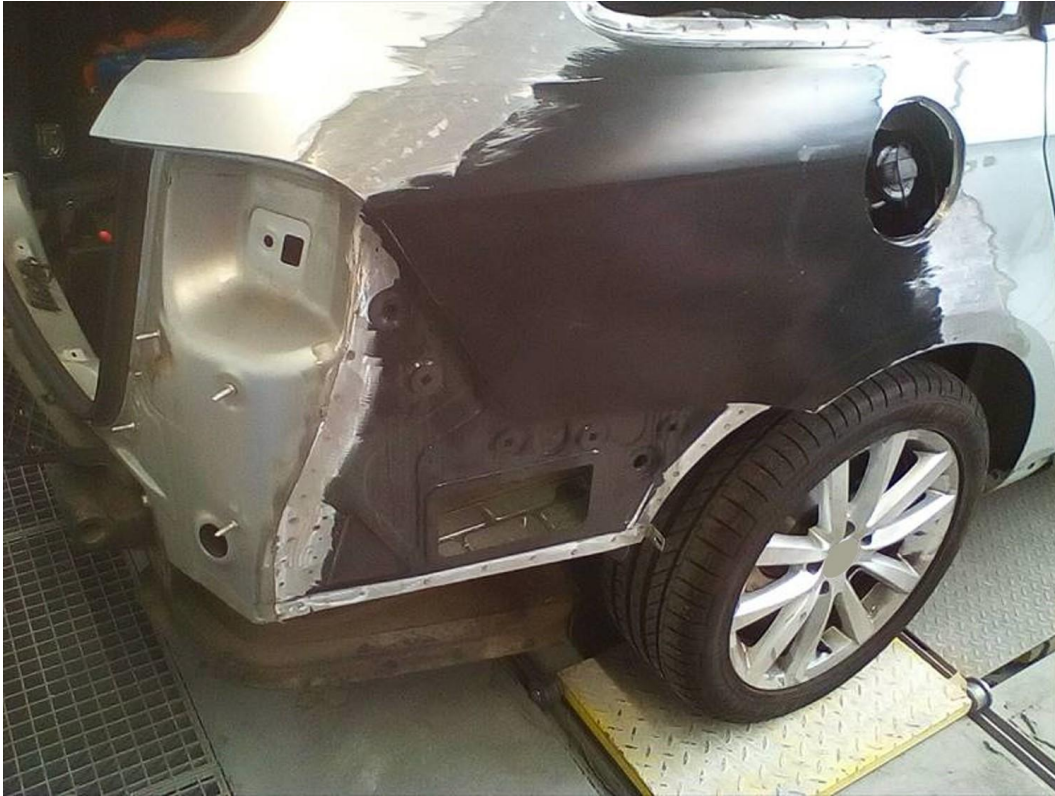
Picture 20: Delivery condition not achieved, mainly caused by missing smooth transition areas from new part to existing body and missing final grinding.
