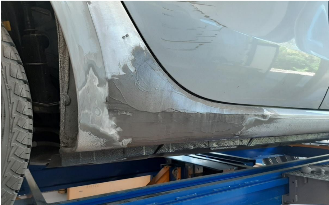
Picture 3: Sill / dog leg after application of 2K epoxy resin body filler.
