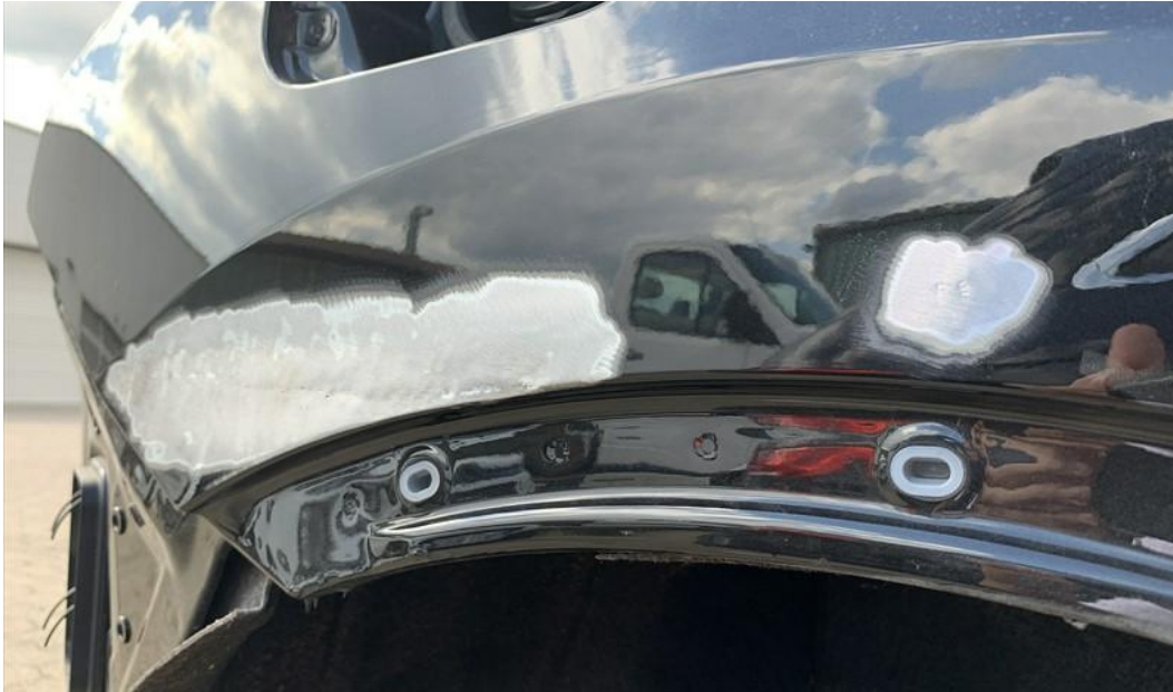
Picture 17: Delivery condition not achieved as repair work is comparatively coarse and imprecise with deep scratches in sheet metal and adjacent paint and a missing smooth transition area to the existing paint
