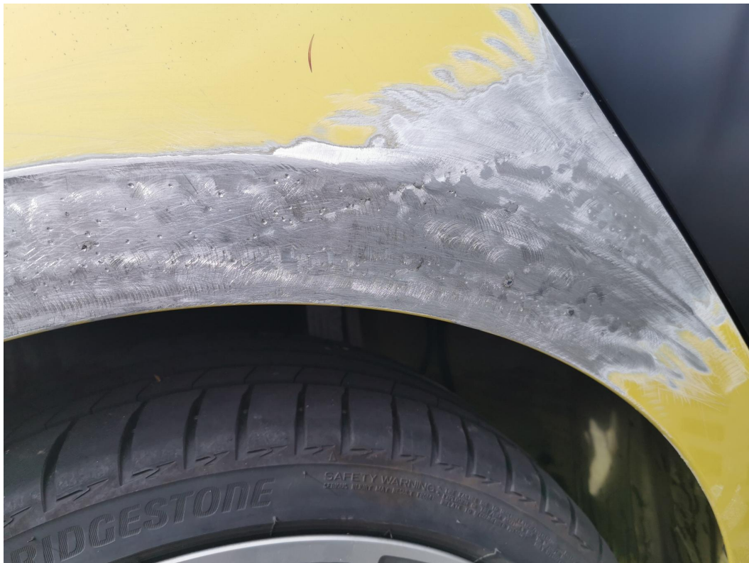
Picture 19: Delivery condition not achieved due to high roughness and missing smooth transition area resulting from a missing final grinding.
