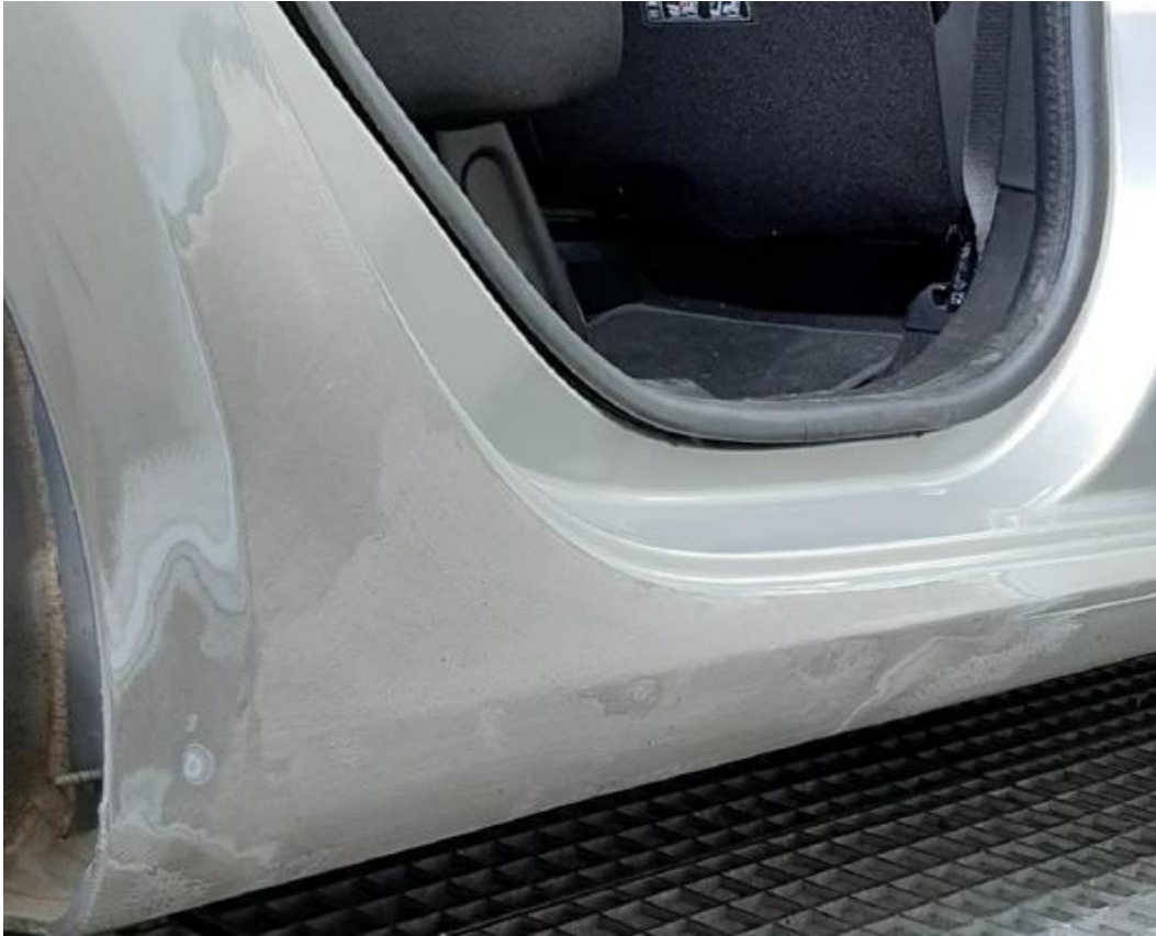
Picture 4: Defined delivery condition achieved after sanding the 2K epoxy resin body filler.
