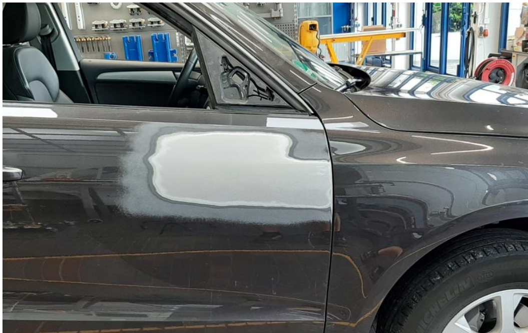
Picture 9: Defined delivery condition achieved without application of 2K epoxy resin body filler.
