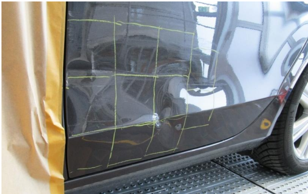
Picture 10: Damaged area as given to the repair shop – example 4.
