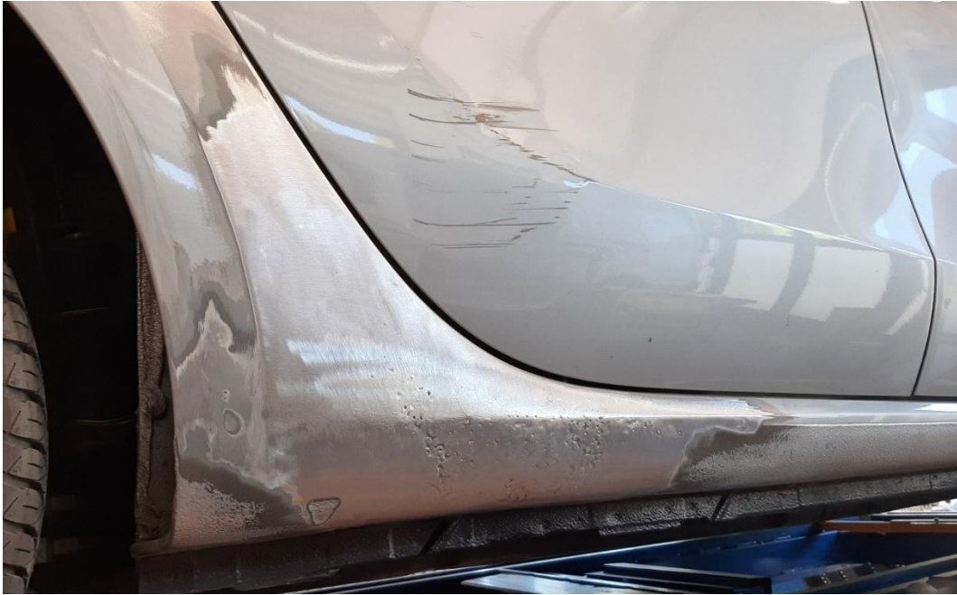
Picture 2: Sill / dog leg after sheet metal repair and before applying 2K epoxy resin body filler.
