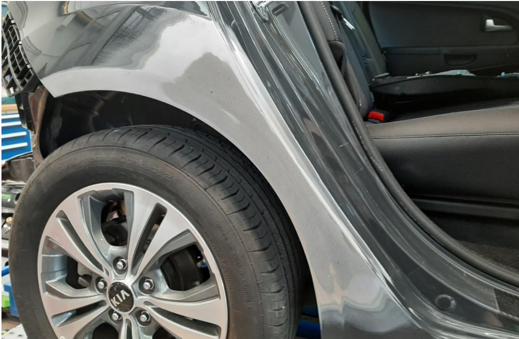
Picture 7: Defined delivery condition achieved after sanding the 2K epoxy resin body filler.
