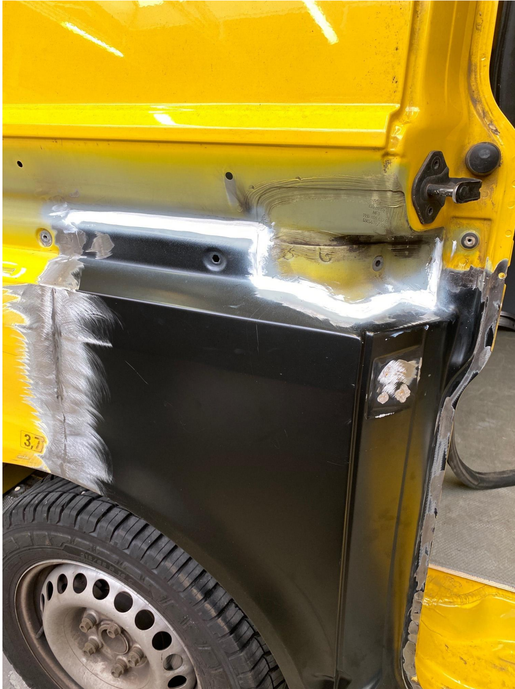
Picture 21: Delivery condition not achieved due to unsmooth transition area and high surface roughness resulting from a missing final grinding.
