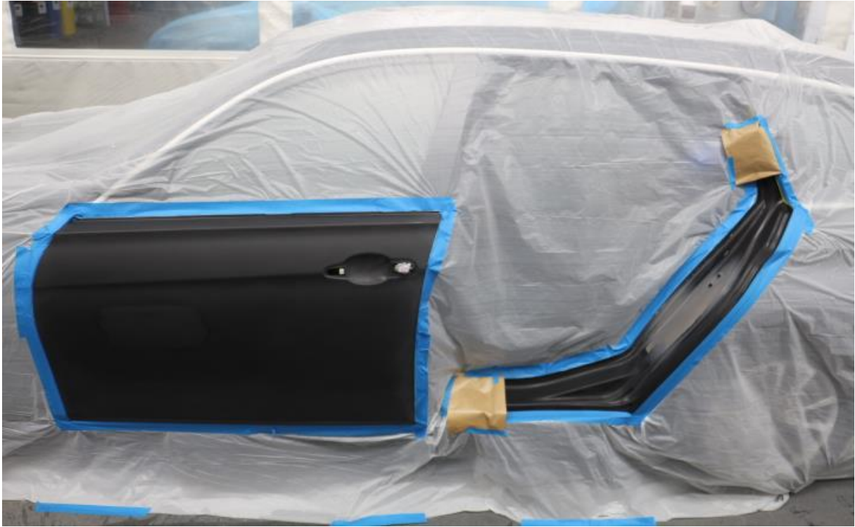
Figure 4: Vehicle prepared for topcoat with repair painting of the rear inner sill section by the fading out painting process on the lower entry sill and along the inner C-pillar.
