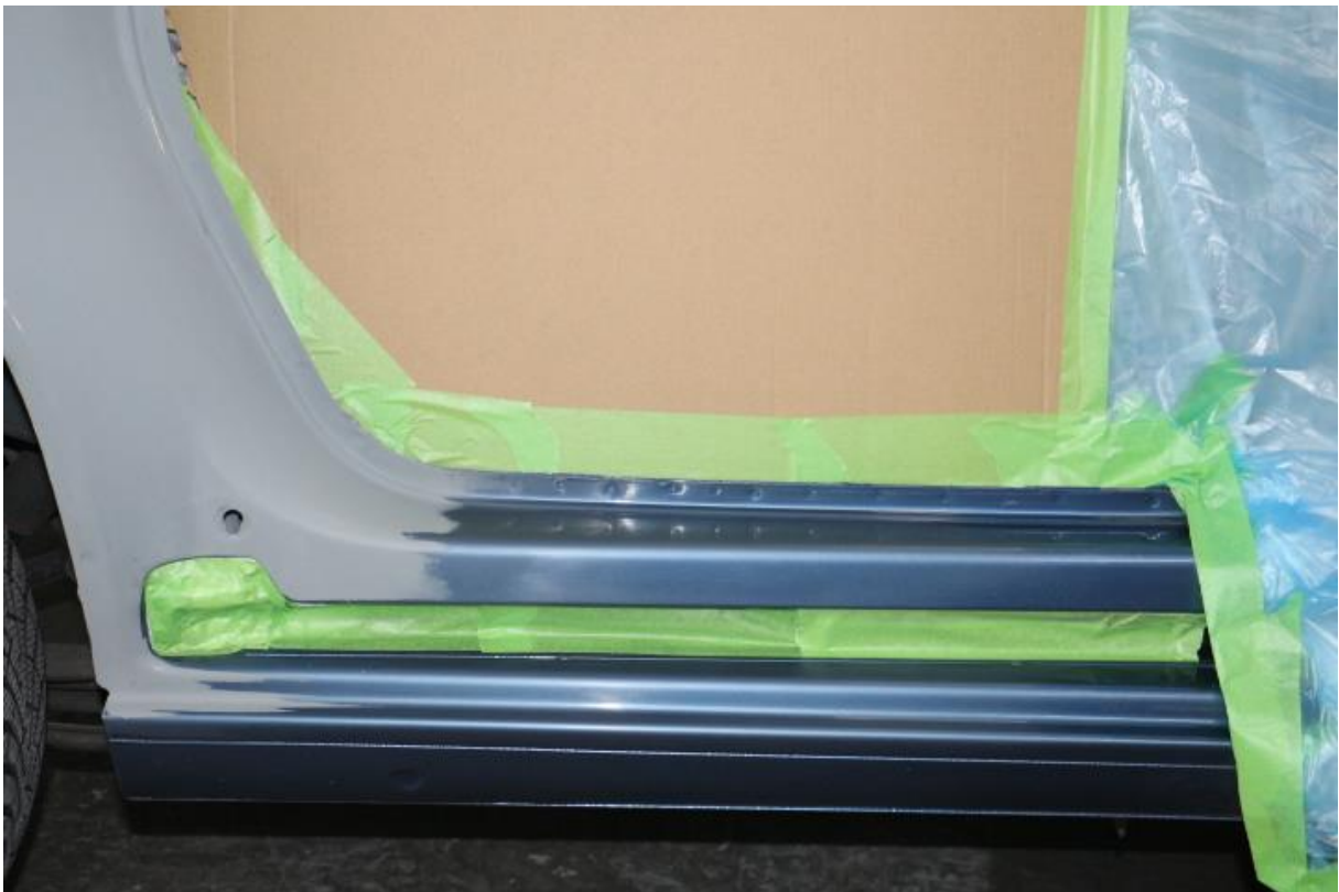
Figure 5: Detailed view of the rear sill section prepared for topcoating using the fading out painting process.
