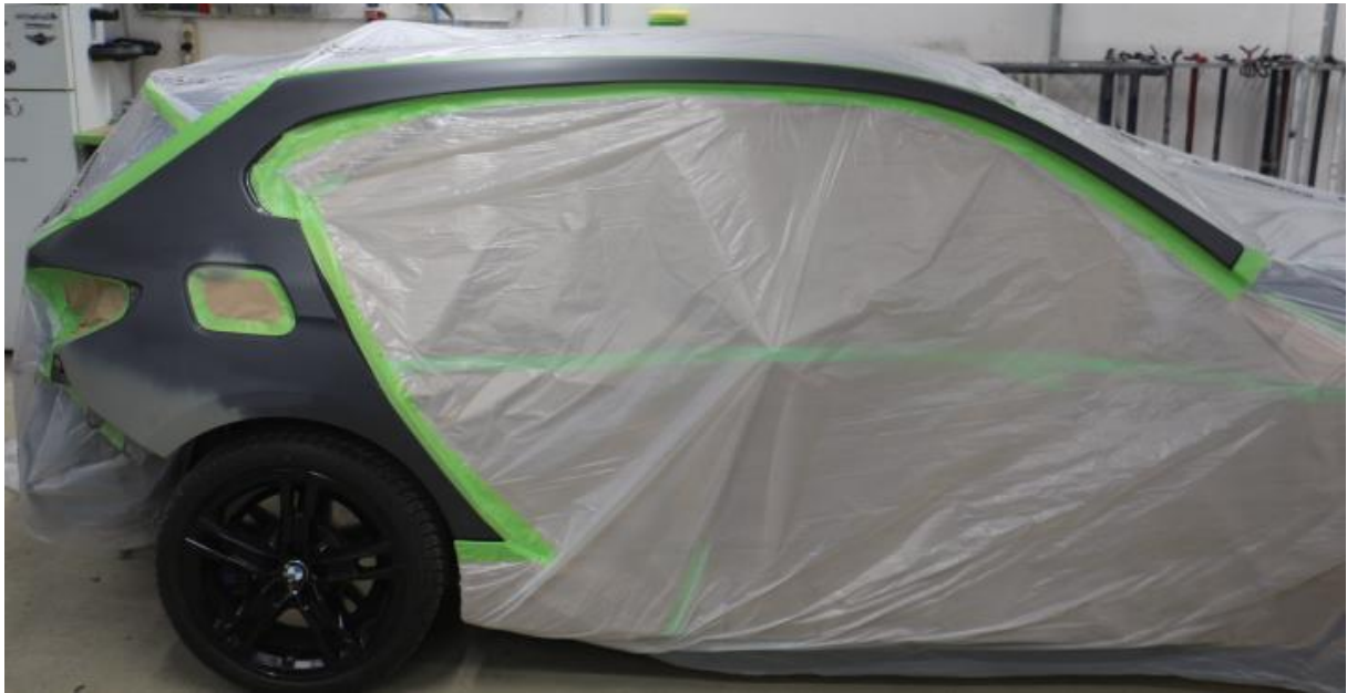
Figure 2: Vehicle prepared for topcoat with repair painting of the rear side panel and supplementary painting of the A-pillar at the top outside to achieve a closed clearcoat.
