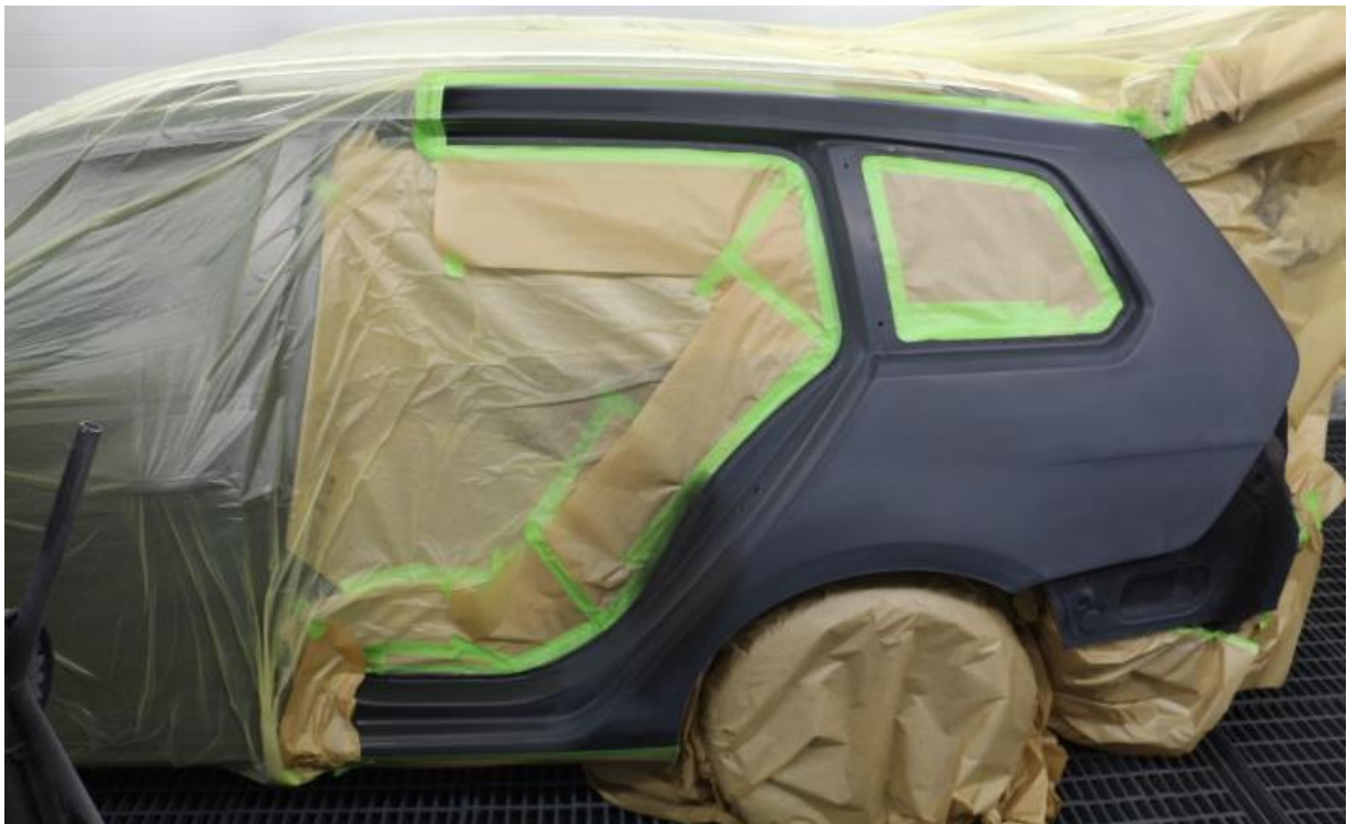
Figure 3: Vehicle prepared for topcoat with repair paint on rear side panel and fading out painting process on roof rail and rear entrance sill area.
