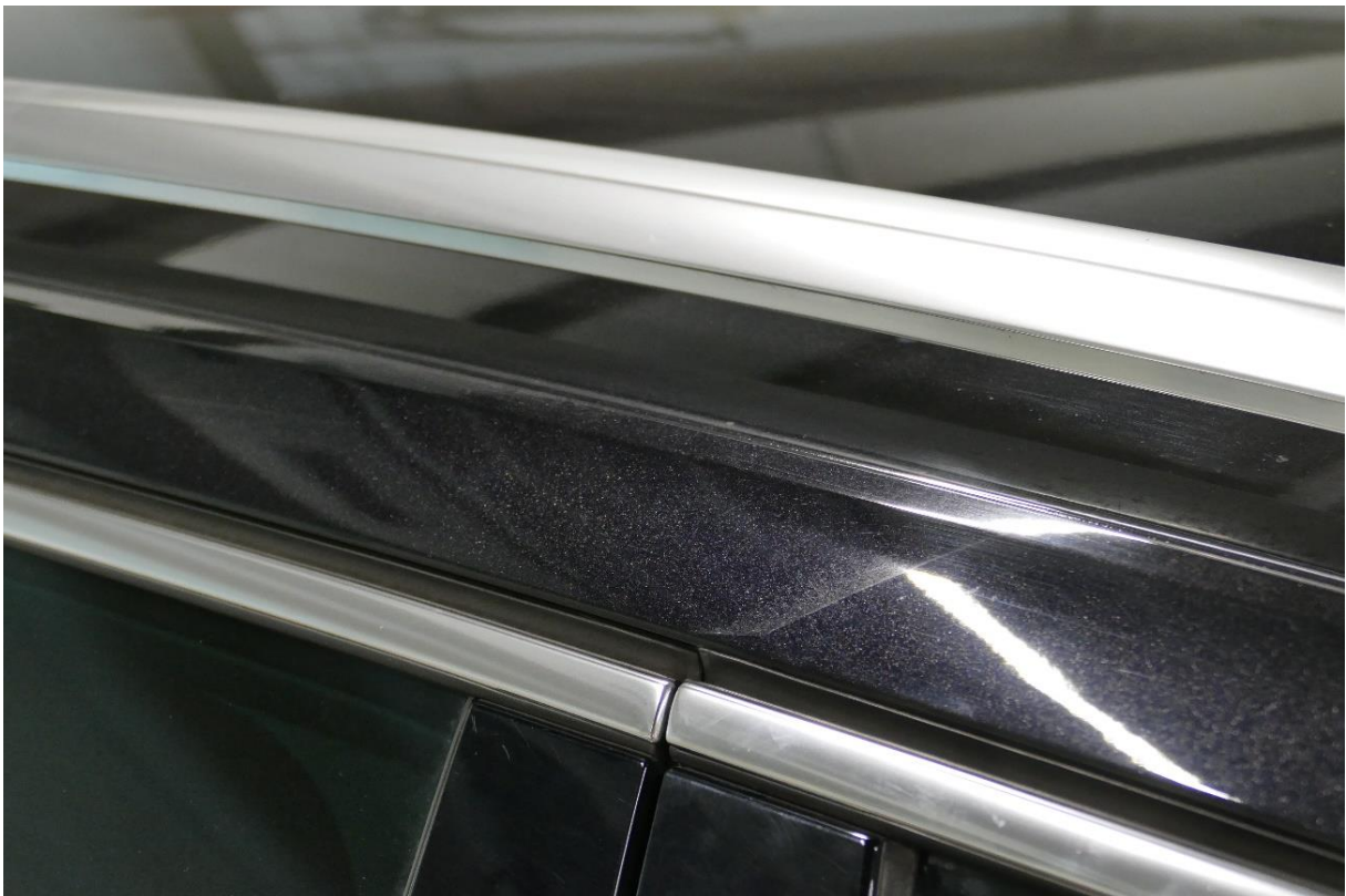
Figure 7: Example of a sharp paint edge due to improper performance of the fading out painting process - transition area not sufficiently dimensioned and subdivided.
