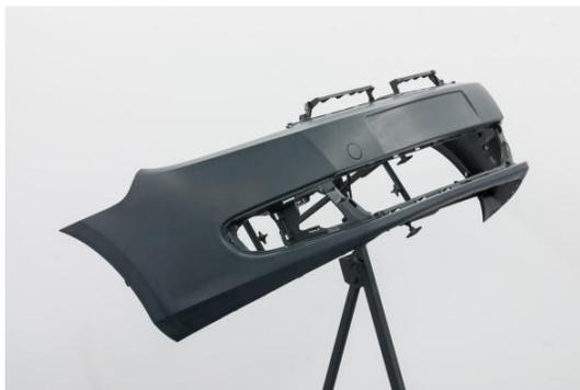
**Remark:** If a different substrate color shade is recommended by the paint manufacturer and a 2-K plastic primer filler in the appropriate gray shade must therefore be applied using the so-called “wet-on-wet”-process, this no longer corresponds to paint stage K1R, but to paint stage K1N.
