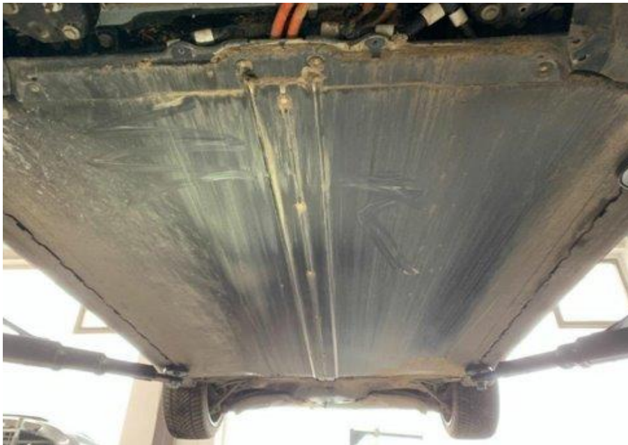
Figure 3: Example of paint damage to be repaired on HV battery
