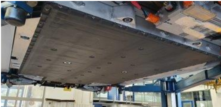
Figure 1: Example of replaceable battery protection, as installed e.g. at VW and Audi
